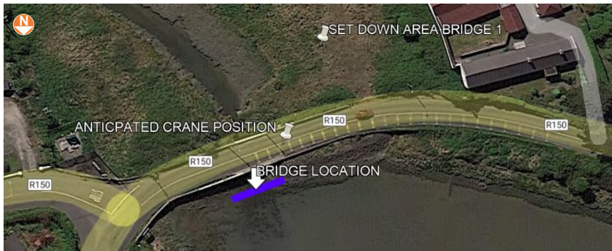
Figure 4-4 Layout for Delivery and Installation of Large Bridge
