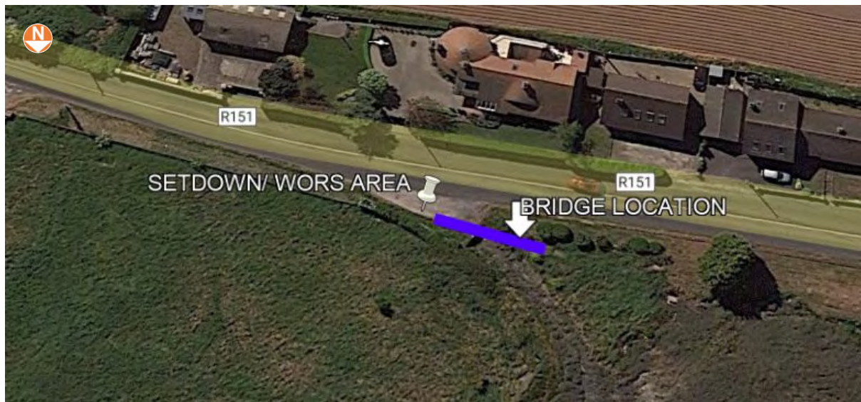
Figure 4-6 Layout for Delivery and Installation of Small Bridge
