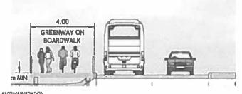
It is recommended that the railing of the boardwalk be set back further from the edge of carriageway.
