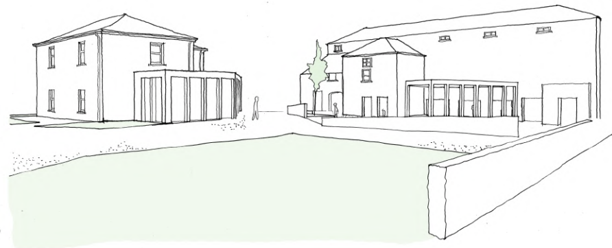
Concept Sketch: showing new single storey intervention to former Bakery Office Building (LHS) maintaining primary elevations to the south and east. Original massing of Corn Store/Mill building becomes legible from Boyne Road and The Ramparts.
