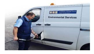
A trial using HVO (Hydrated Vegetable Oil) has commenced and is now two months into implementation. The trial incorporated 10 vehicles from our Transportation, Environment and Civil Defence sections. It is a direct replacement fuel for diesel engines with a 90% reduction in CO2
