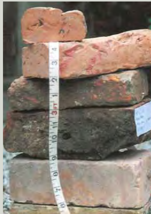
The changing sizes of brick: this image shows, from the top, the thin bricks of the seventeenth century, an eighteenth-century handmade brick and a nineteenth-century machine-made brick
