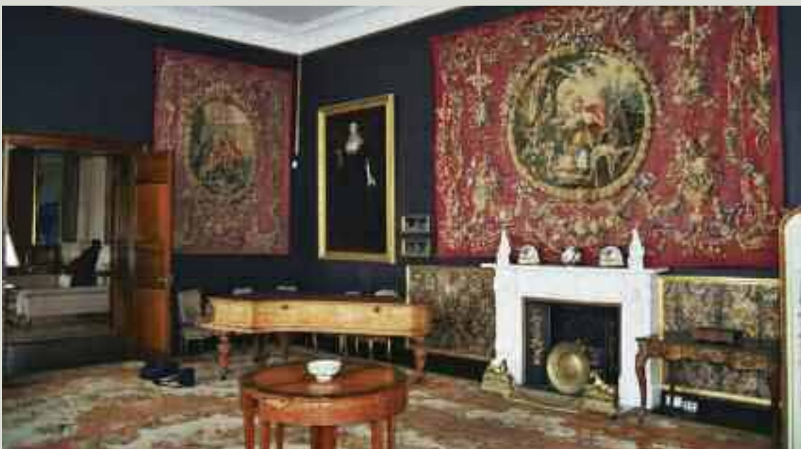
Leather linings and tapestries line the walls of this room and improve the thermal comfort of the occupants
