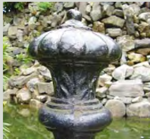
Castings should be checked before they are put in place to ensure that they are of acceptable quality. The casting illustrated above is deformed because the two halves of the mould were not aligned correctly during the casting process
