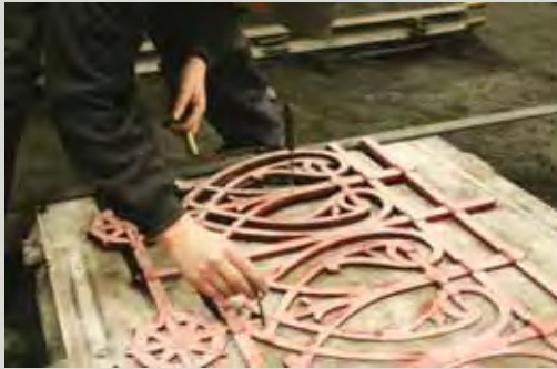
Green sand moulding is a highly skilled craft. This image shows a timber pattern being removed from one half of a green sand mould (Image courtesy of Historic Scotland and Charles Laing & Sons, Edinburgh)
